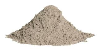
used construction materials in the world. Our Type IL is branded as **EcoCem®** *PLC* and was developed to be more environmentally friendly by reducing its carbon footprint (reduction measured through GWP). This product is a general use product for concrete and mortar as well as all the other various applications for cement, including engineered soils and solidification/stabilization of materials and wastes.
