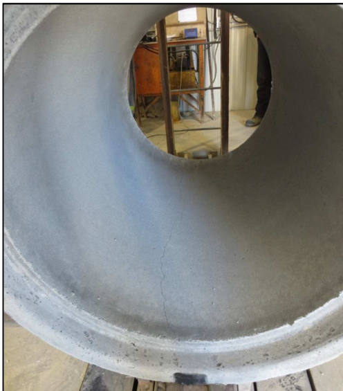
Figure 4 (above): RCP Displaying Shear Failure
