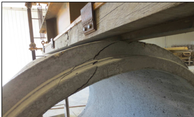
Figure 3 (left): Flexural Failure in Three-Edge Bearing Machine Test
