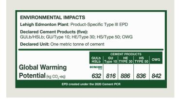
EcoCem®PLUS is an innovative blended portland limestone cement (PLC) designed to provide strength and durability while significantly reducing carbon footprint in concrete.
